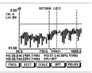
Figure 3-5. Cable Return Loss Measurement Results
