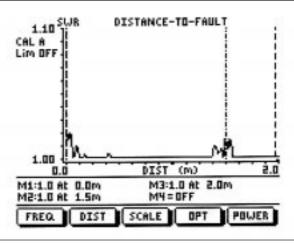
Figure 3-11. DTF-SWR Measurement Results (Cable Quality)
