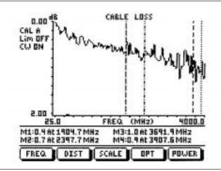
Figure 3-7. Cable Loss Measurement Results
