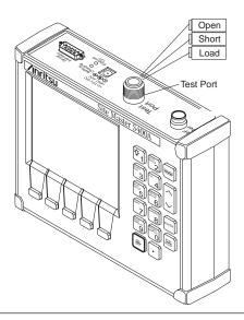
Figure 3-1. Measurement Calibration Test Setup
