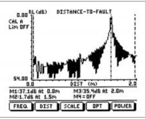
Figure 3-8. DTF-Return Loss Measurement Results (Cable Length)
