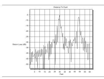
Figure 2-4. Rectangular Windowing Example
