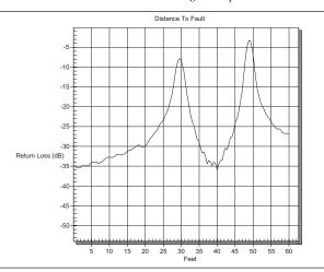
Figure 2-7. Minimum Side Lobe Windowing Example
