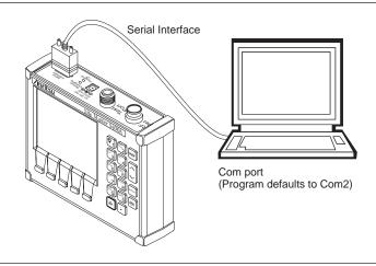
Figure 4-3. Equipment Setup for Site Master Tools Operation
