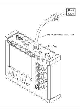
Figure 3-4. Cable Measurement Test Setup
