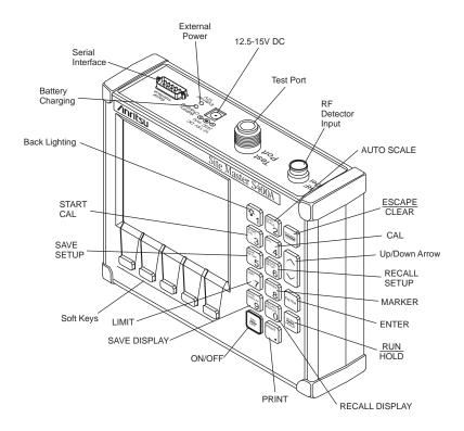
Figure 2-1. Site Master Controls and Connectors
