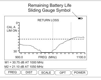
Figure 2-8. Battery Monitor
