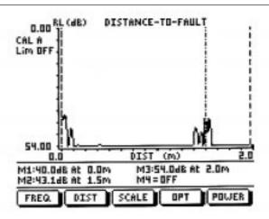
Figure 3-10. DTF-Return Loss Measurement Results (Cable Quality)
