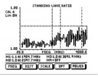
Figure 3-6. Cable SWR Measurement Results
