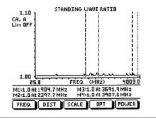
Figure 3-3. SWR Measurement Mode Calibration Results
