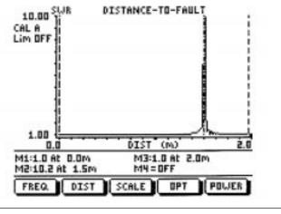
Figure 3-9. DTF-SWR Measurement Results (Cable Length)
